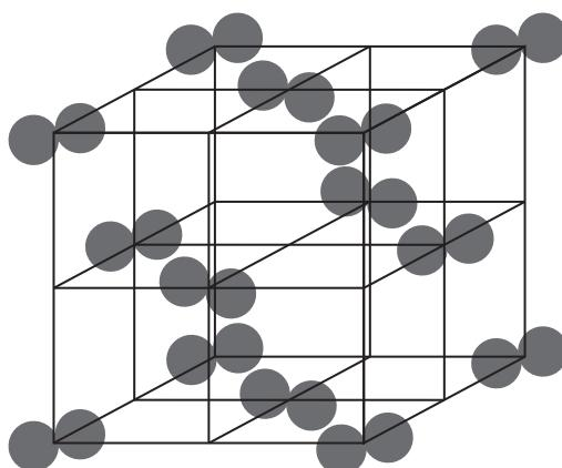
Each iodine molecule is held in place by weak intermolecular forces.
